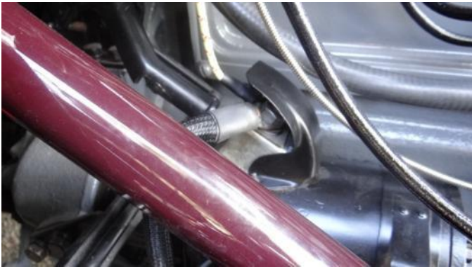
Genuine factory shroud to insulate the starter motor switch.
