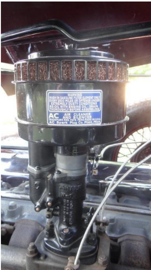
W-1 Carter Downdraft Carburettor.
