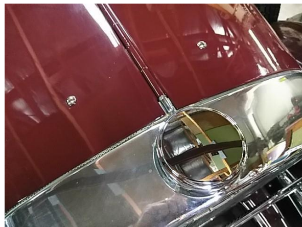
Unique to Australian 1932 Chevrolets were 2 chrome half-domes on each side of the bonnet which meet when the bonnet is opened.
